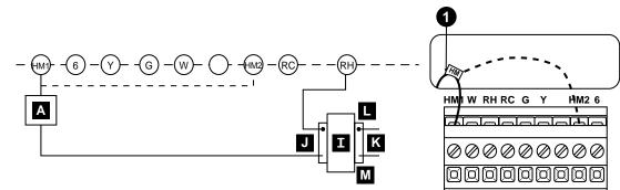
NOTE: Two terminal choices (**HM1** or **HM2**) are provided for humidifier control. When the humidity setting is higher than the room humidity:
